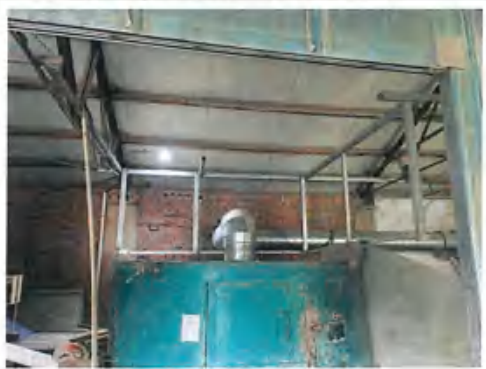
镁质耐火材料搅拌集气罩
